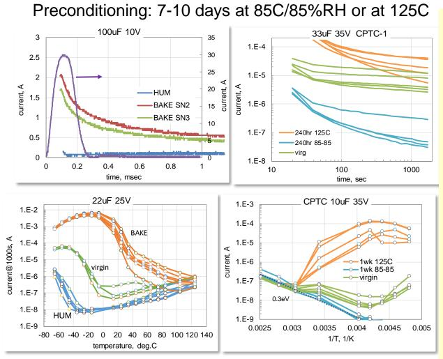
Preconditioning affects transient currents from 0.1 millisec to hours. Behavior of CPTCs with moisture is similar to MnO2 caps. ✓ At RT dry CPTCs might have currents >10<sup>3</sup> times greater than humidified caps. Contrary to MnO2 capacitors, leakage currents at low
