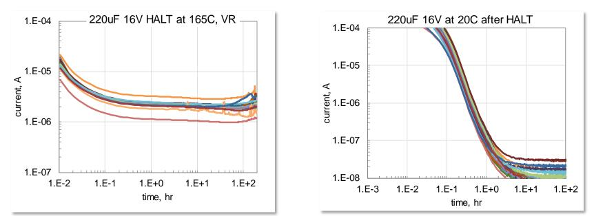
✓ Currents at RT after HALT during first few minutes exceeded currents at 165 °C by orders of magnitude and then decreased more than 10<sup>4</sup> times after 10 hours.
