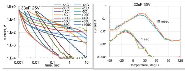
Anomalous transients appear in vacuum after ~100hr. Currents might exceed 1 mA for more than 5 min. Inverse temp. dependence of leakage currents. Short- and longterm transients have different extremal dependencies on temperature and might be due to different mechanisms.
