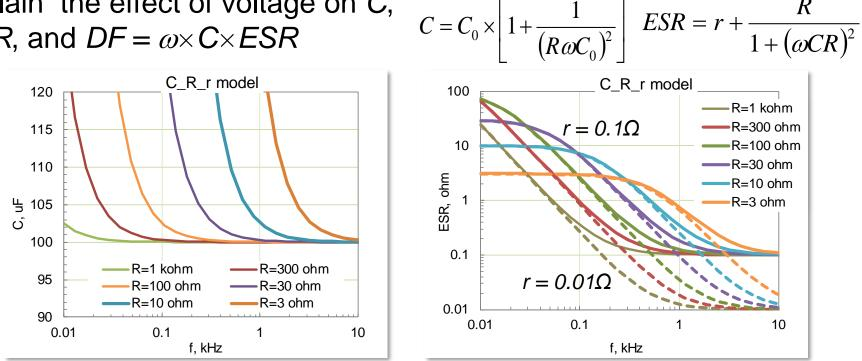
The effect is due to increased conductivity of Ta2O5 that increases sharply with voltage.
