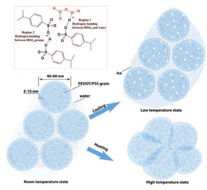
Changes in morphology of PEDOT/PSS with moisture content and temperature, Zhou et al. 2014
