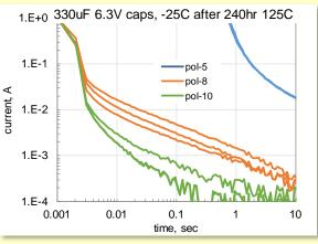
Transient currents are increasing at low temperatures and might exceed 1A for up to 1 sec that might be interpreted as a short circuit failure during cold start-up of the system.
